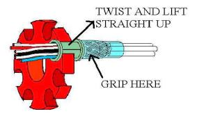
For maximum contact extraction tool access, unclip all ferrules from the star, remove the star from the cable bundle before pushing the adapter body (4) toward the cable.
