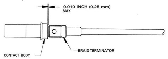
• The solder must have completely melted and flowed through the holes in the braid terminator body and into the braid strands underneath. The solder must form an acceptable fillet (75%) in a minimum of one inspection hole (not all holes must show an acceptable solder joint).
