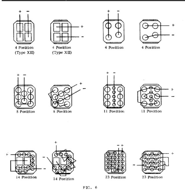
Wiring Diagram, Suggested Method for Insulation Resistance and Dielectric Strength Tests
