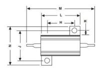
**HSA5 - HSA10** : Mounting Hole 2 x 2.4mm **HSA25 - HSA50** : Mounting Hole 2 x 3.3mm
