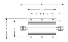
**HSC200 - HSC250** : Mounting Hole 2 x 2.4mm **HSC300, HSHC350 - HSHC500** : Mounting Hole 2 x 3.3mm
